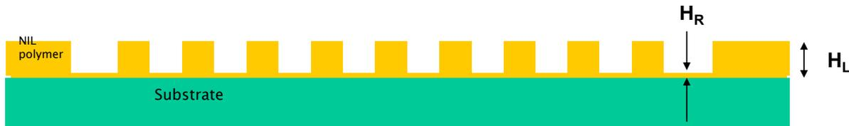
Figure 14. Residual NIL polymer after stamping step
