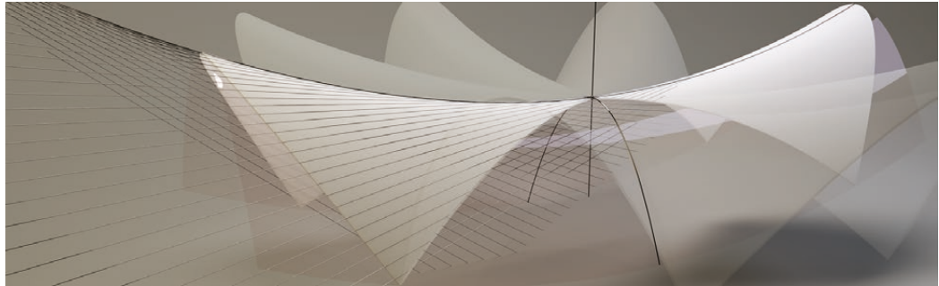
Fig. 1. Hyperbolic paraboloid and its sections in the Los Manantiales Restaurant by Felix Candela (Mexico City, 1956).
