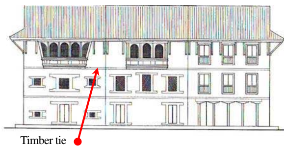
Fig 3: Symmetric residences with timber ties on wall
