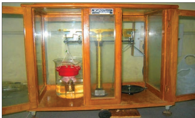
Figure 1: Experimental set up for bioadhesive strength
