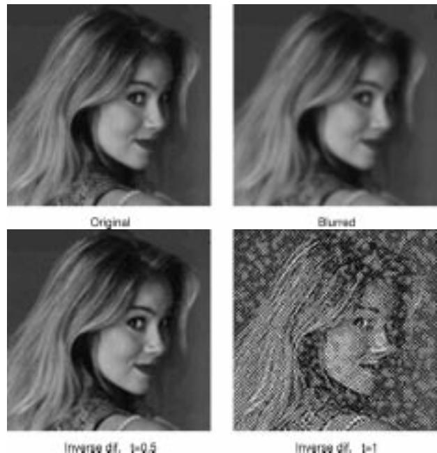
Fig. 2. Two-dimensional linear inverse diffusion. From top left (clockwise): original image, blurred, inversely diffused at times 0.5, and 1, respectively.
