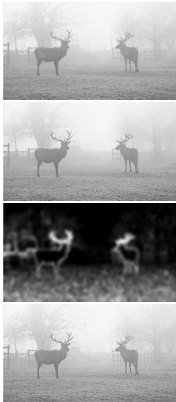
Fig. 11. FAB diffusion process applied to the deer image. From top: original image, result of processing with constant parameters k_f = 2 , k_b = 50 , w = 10 ; magnitude of smoothed gradient of original image T(x, y) = |\nabla I_0 * G_\sigma| , ( \sigma = 3 ); result of processing with spatially varying parameters k_f(x, y) = 0.1T , k_b(x, y) = 6T , w(x, y) = 2T .
