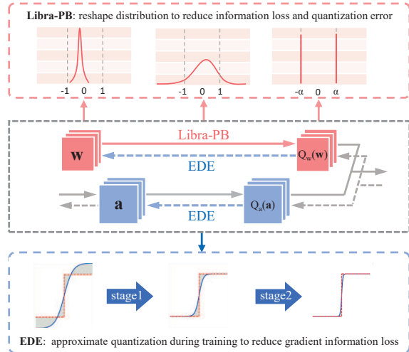
Figure 1: Overview of our IR-Net training for a convolutional layer, consisting of Libra Parameter Binarization (Libra-PB) in forward propagation and Error Decay Estimator (EDE) in backward propagation. Libra-PB changes the weight distribution in forward propagation to retain the information of weights and activations. And the shape change of EDE during the entire training process reduces the gradient information loss in backward propagation.
