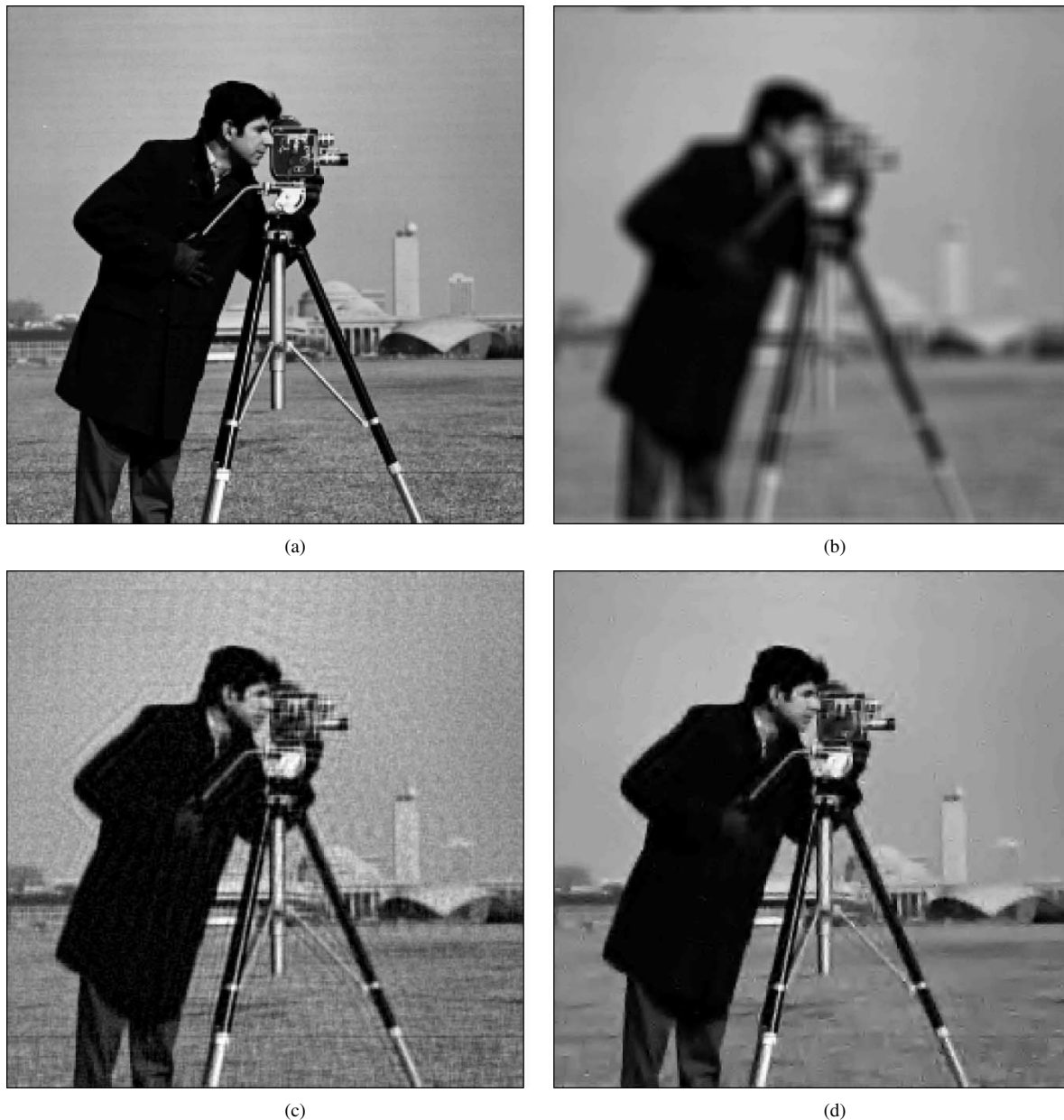
Fig. 4. (a) Desired Cameraman image x ( 256 \times 256 samples). (b) Observed image y : x smoothed by a two-dimensional (2-D) 9 \times 9 box-car blur plus white Gaussian noise with variance such that the BSNR = 40 dB. (c) LTI Wiener filter estimate (SNR= 20.8 dB, ISNR = 5.6 dB). (d) ForWaRD estimate (SNR = 22.5 dB, ISNR = 7.3 dB). See Section VIII for further details.
