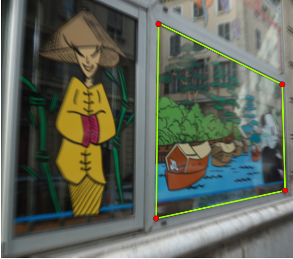
Figure 5. Illustration for finding vanishing lines. Two sets of parallel lines on a blurred plane are drawn to find two vanishing points. It is easy to locate parallel lines based on scene structure by humans.
