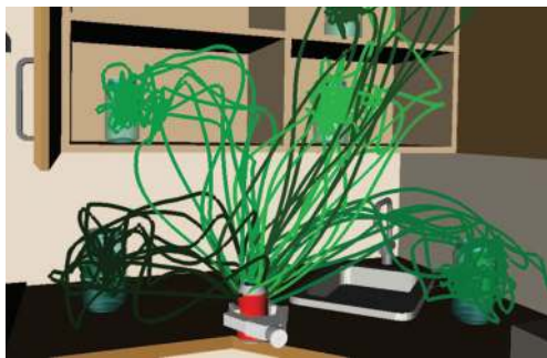
Figure 2. A subset of the possible end-effectors path for a shared control assistive arm in daily life activities. (Image courtesy of RoboticsLab, UC3M.)
