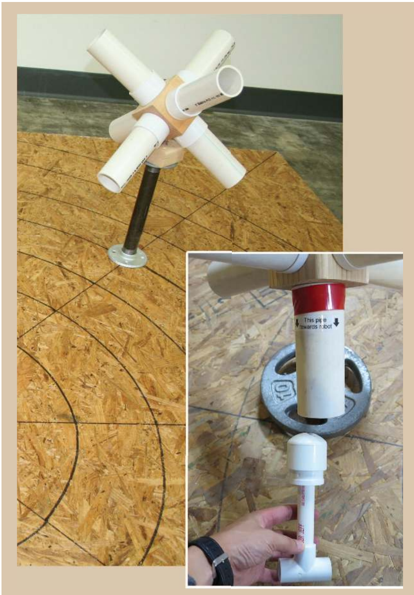
Figure 3. The nodal apparatus for a manipulator dexterity evaluation. This model has six directed inspection targets and can be used for retrieval and insertion evaluation as well. (Image courtesy of NIST.)
