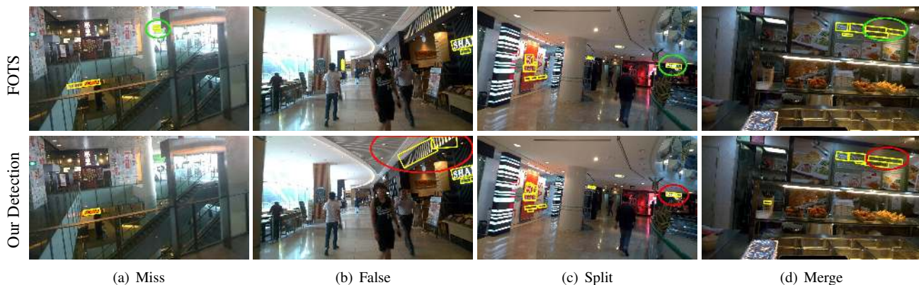
Figure 5: FOTS reduces Miss, False, Split and Merge errors in detection. Bounding boxes in green ellipses represent correct text regions detected by FOTS, and those in red ellipses represent wrong text regions detected by “Our Detection” method. Best view in color.
