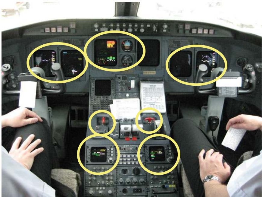
Fig. 4.13 The use of color and luminance on aircraft displays facilitates the finding of particular information (this will be less apparent in b/w versions of this figure!)
