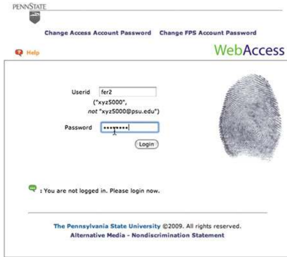
Fig. 2.2 An example interface that attempts to “fit the user to the machine”. In the top entry field the user is expected to remove the domain rather than have the system do that (many sites, including Gmail, will let users login with either user-name or user-name@domain, this one does not)
