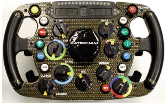
Fig. 3.1 The steering wheel from the Caterham 2012 Formula 1 car. The wheel contains multiple controls to adjust traction, suspension, and aerodynamics (reproduced with permission of Caterham F1 Team, UK)
