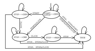
Figure 1: Automaton for the mouse program
