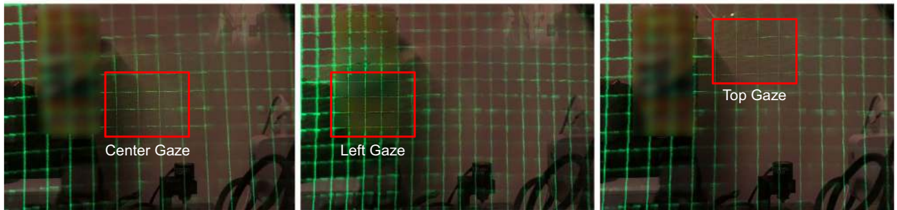
Figure 4. Demonstration and implementation of the foveated near-eye display. (a) Schematic diagram and a photograph of the benchtop prototype. (b) Experimental result to show the resolution enhancement in the foveal region. We compare two experimental results where the foveal display is on or off. (c) Demonstration of optical steering the viewing window of the foveal display using the MEMS mirror. Optical steering results for horizontal and vertical direction are presented. Note that the resolution enhancement by the foveal display is more significant than the demonstration in these photographs. The photographs are captured by a mobile phone camera where the maximum angle resolution is less than the resolution limit of the foveal display (30 cpd). Due to copy right permission, we blurred portion of the image.
