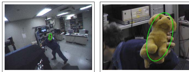
Fig. 5. Maintaining the object view in foveal image based on information from the peripheral view
