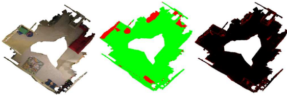
Figure 10: Relationship between accuracy and curvature. Left: raw point cloud. Middle: prediction of FPCConv with incorrect points highlighted in red, and correct in green. Right: points with large curvature are highlighted in red. We can see that distribution of incorrect points is consistent with large curvature points.
