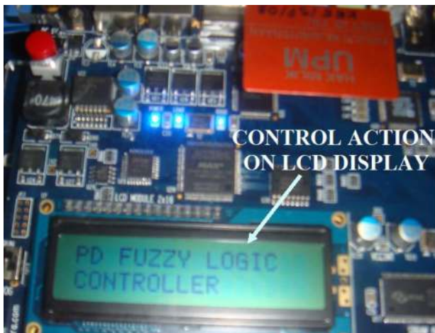
Fig. 15: LCD display in DE2 board.
