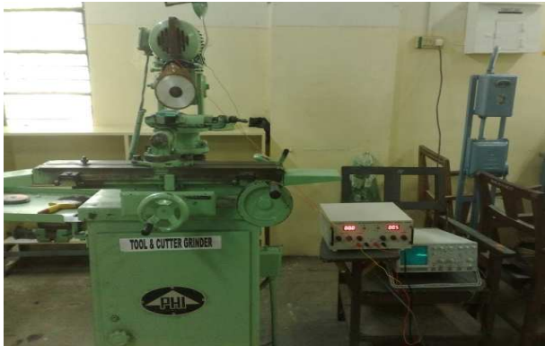
Figure 3. Experimental setup of grinding process.
