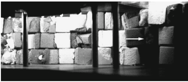
Fig. 7 View into the “A” channel of the model. Image taken by the black and white high speed camera during the experiment. The arrow indicates the flow in the x' -direction and serves as a scale. Its length is 32 mm, which equals the initial side length r_0 of the intact blocks. The rock blocks remain in contact during the entire experiment. This simulation was performed at an angular velocity \omega of the centrifuge of 30.4 rad/s
