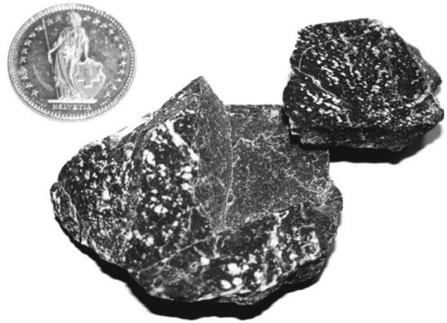
Fig. 4 Chunks of massive, micritic Malm limestone sampled from the sturzstrom of Flims. This sample is representative of the angularity of particles forming in sturzstroms—independent from their diameter and geology. The rough fracture surfaces are not pre-existent in the source rock but are newly formed by fragmentation during the transition of the sturzstrom. These two chunks fit together like a “jigsaw puzzle” [114, 115]. The white spots are lunette shaped impact marks by other rocks, but no signs of abrasion are observable (a 27 mm dia. coin serves as scale)
