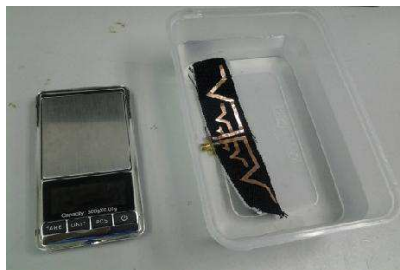
Figure 13. Antenna are tested under wet conditions.
