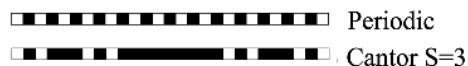
Fig. 1. Periodic and fractal 1-D structures to be used to generate zone plates.
