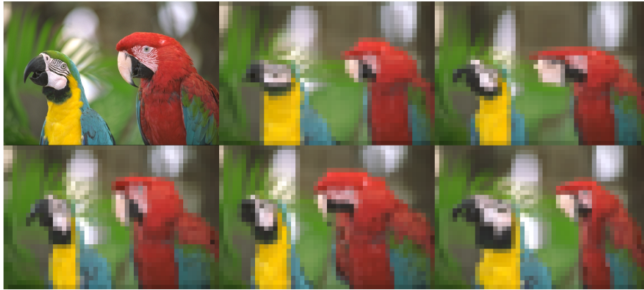
Figure 2: Top left, ‘Kodak True Color’ parrots at a resolution of 384 \times 256 . The other five images are one-eighth of the resolution as a result of 6 layers of average pooling using disjoint random FMP \sqrt{2} -pooling regions.
