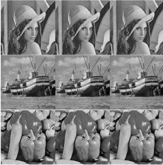
Fig. 1. From left to right, the noisy image with \sigma = 15 , the reconstructions with respectively Bai and Feng's algorithm [1] and Algorithm 1, the fractional order \alpha is equal to 1.5. From top to bottom, the Lena, Boat and Peppers images.
