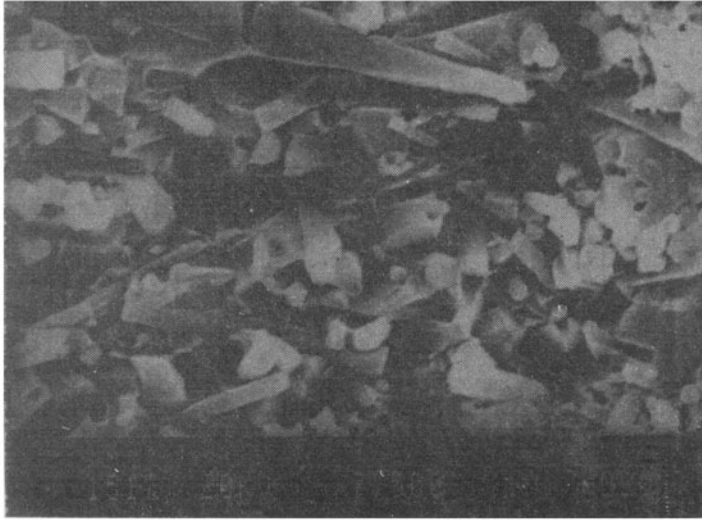
Figure 10. At high \Delta K region, the alumina grains failed in a mixed mode i.e. intergranular (~ 45%) and transgranular (~ 55%).
