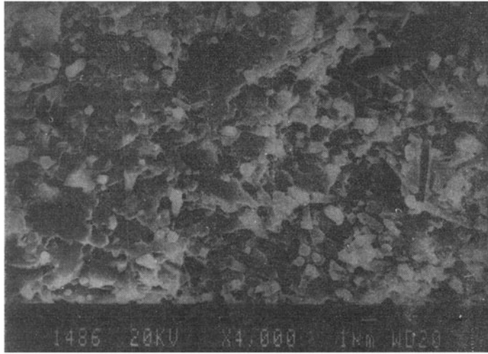
Figure 6. At low \Delta K (0.8 to 1.8 \text{MPa}\sqrt{m} ) region, a majority of the whiskers failed with a square fracture without evidence of large scale pullout.
