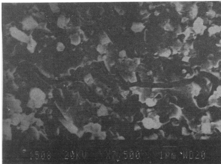
Figure 13. Crack deflection in the low \Delta K region.
