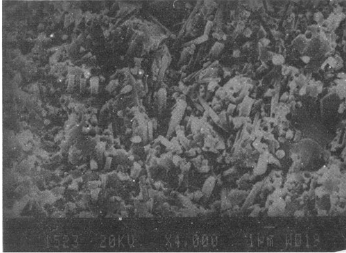
Figure 8. In the fast fracture region ( K_{IC} = 5.9 \text{ MPa}\sqrt{\text{m}} ), whiskers failed predominantly by pullout mechanism.
