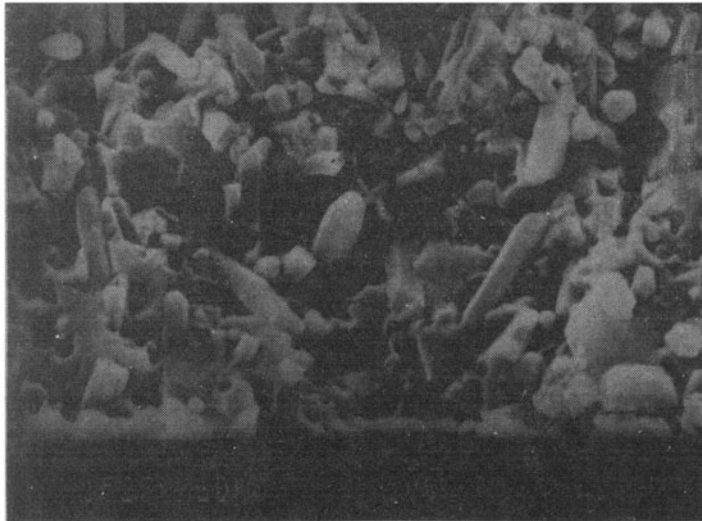
Figure 11. In the fast fracture region (monotonic loading), the alumina grains failed in a mixed mode, i.e. intergranular (~ 55%) and transgranular (~ 45%).
