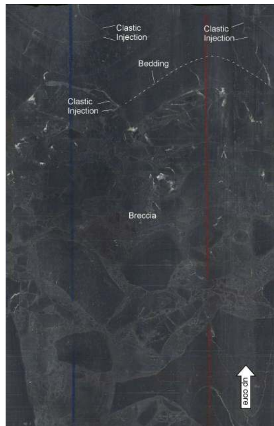
Fig. 11 – Whole-round CoreScan II™ image of a 'jigsaw' breccia with clastic injections both across and along bedding at 1233.56 mbsf in the AND-1B core. Core is 4.5 cm in diameter.
