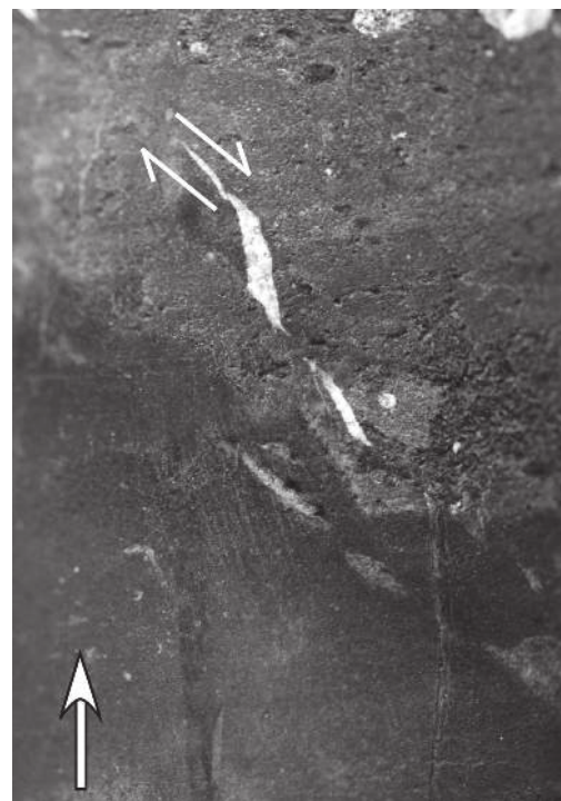
Fig. 15 – Photograph of calcite-filled pull-aparts indicating normal-sense fault displacement at 1173.62 mbsf in the AND-1B core. Core is 4.5 cm in diameter. Arrow points upcore.
