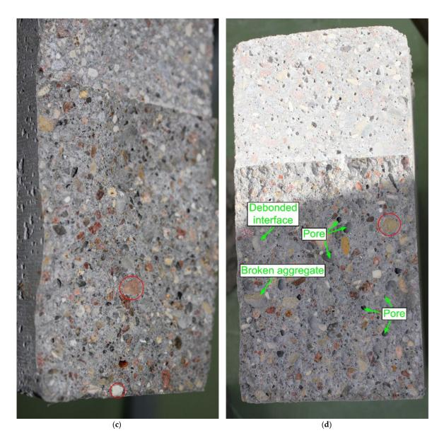
**Figure 4.** Cross-section of the analyzed concrete composites after a fracture toughness test, with visible characteristic macroscopic structure: (a) REF, (b) QBC-1, (c) QBC-2, (d) QBC-3.
