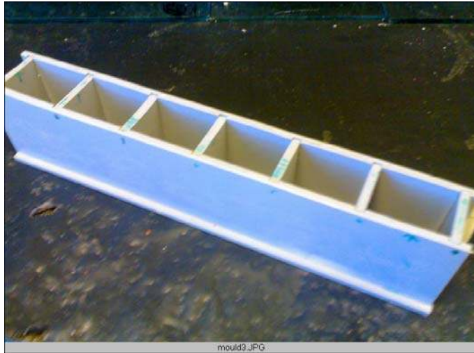
Figure 5: The mould for short bar specimens
