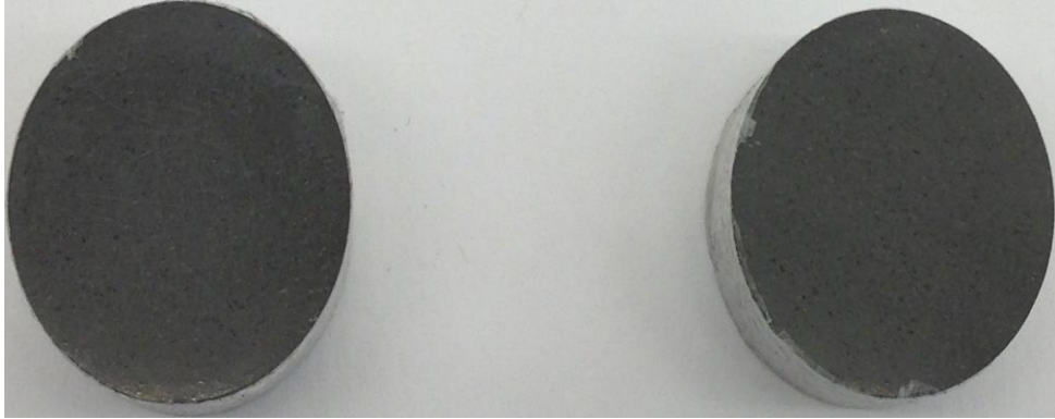
Figure 4.29: Images of bottom (left) and top (right) cores from Freshwater Test#1 without any pressure or proppant effect. Core diameters are 1.0 inch.
