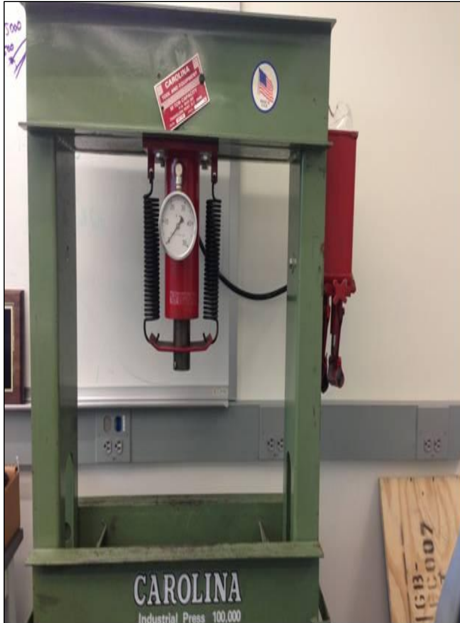
Figure 3.7: Image showing the high pressure press. The steel pipe moves down and applies pressure to any component that is placed on top of the rails. Rods on the right side are cranked, and the steel pipe moves down via the springs. The gauge shows the amount of pressure applied once the steel pipe makes contact with a surface.
