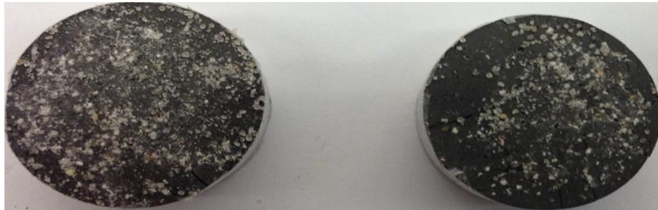
Figure 4.34: Bottom and top cores from Freshwater Test#2 loaded with 20/40 Ottawa at 0.1 \text{ lb/ft}^2 after they were subjected 3030 psi for one hour. Core diameters are 1.0 inch.
