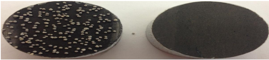
Figure 5.38: Bottom and top cores from KCl+friction reducer Test#1 loaded with 20/40 Ceramic at 0.1 lb/ft 2 (no pressure). Core diameters are 1.0 inch.
