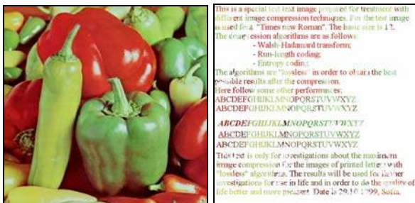
c. Watermarked test image d. Extracted watermark Fig. 7. Example test image “Peppers” (24 bpp, 512 × 512 pixels).
