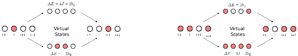
FIG. S1. Virtual second-order processes that give rise to the nearest-neighbor spin exchange.
