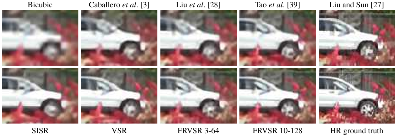
Figure 10: Visual comparison with previous methods on Foliage from Vid4. Amongst prior art, Liu and Sun [27] recover the finest details, but their result has blocky artifacts, and their method uses a slow optimization procedure. Between the remaining methods, even the result of our smallest model FRVSR 3-64 is sharper and contains more details than prior art, producing results similar to the much bigger VSR model. Our larger model FRVSR 10-128 recovers the most accurate image.
