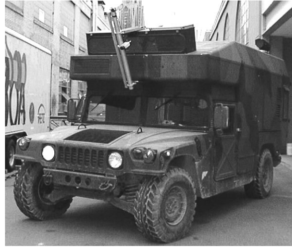
Fig. 7 The autonomous vehicle (HMMWV) that used for our experiments. The vehicle is equipped with stereo vision, inertial guidance and GPS positioning.
