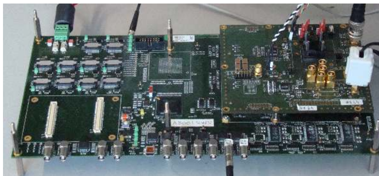
Figure 7: The digital mother board and the analogue mezzanine prototypes described in the text. The A3PE FPGA is visible on the digital part. The analogue part supports the discrete component implementation and the ICECAL ASIC (maintained on the PCB of the mezzanine with the black support at the top right).
