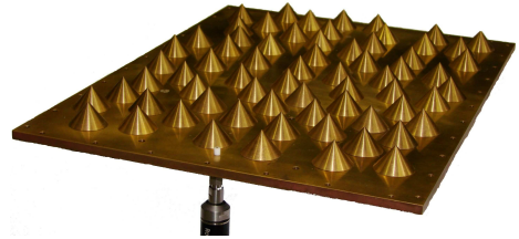
FIG. 1: (Color online) Photograph of one of the two scattering arrangements used. The platform has width 260 mm and length 360 mm. Each cone has diameter 25 mm and height 15 mm. The probe antenna is fixed in a horizontally movable top plate located 20 mm above the bottom (not shown).
