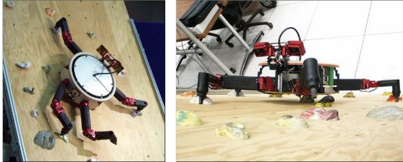
Fig. 1. LEMUR IIb, a multi-use robot capable of free-climbing.
