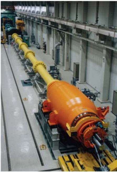
FIG. 1. Free-piston shock tunnel HIEST.
