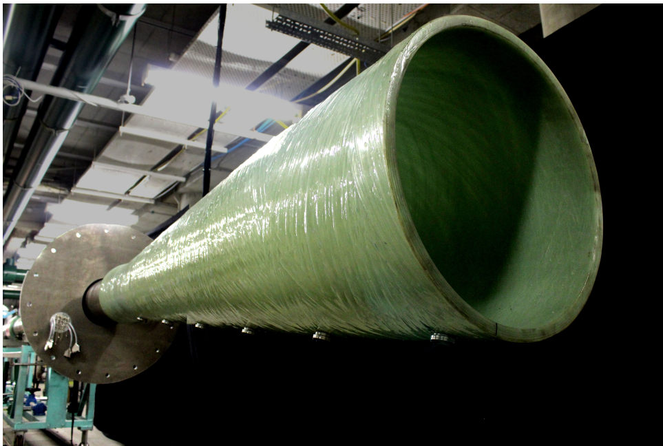
Figure 4.26: The new Mach 12 nozzle installed and cantilevered off the acceleration tube. On the aluminium plate the nozzle instrumentation plate can be noted. On the bottom surface of the nozzle the nozzle sensors mounts are visible.
