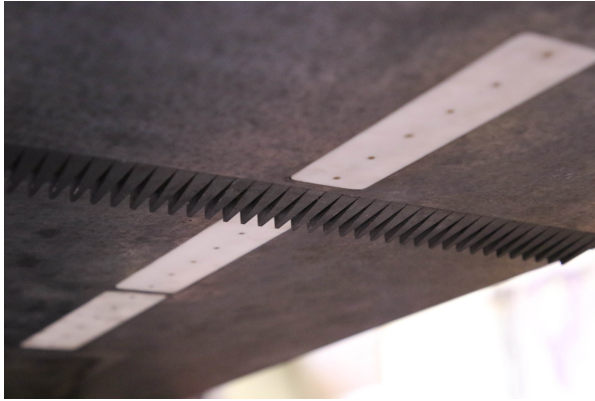
(a) TFHTG installed in the engine forebody
