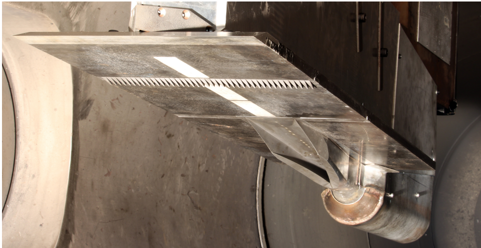
Figure 6.1: Mach 12 Rest engine fully assembled inside the X3 test section. For this picture, swept ramp trip has been used.
