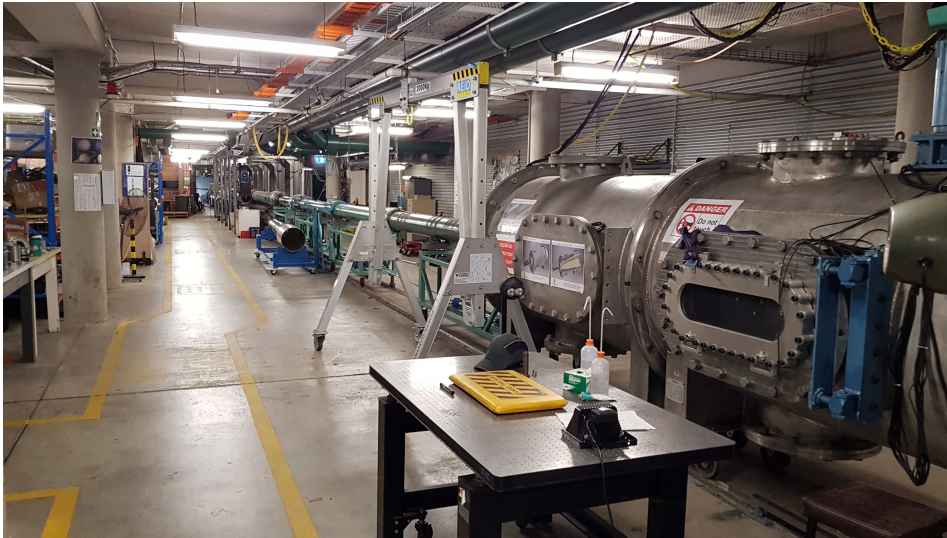
Figure 2.16: X3 expansion tube inside the expansion tube laboratory. In the foreground the test section and dump tank.
