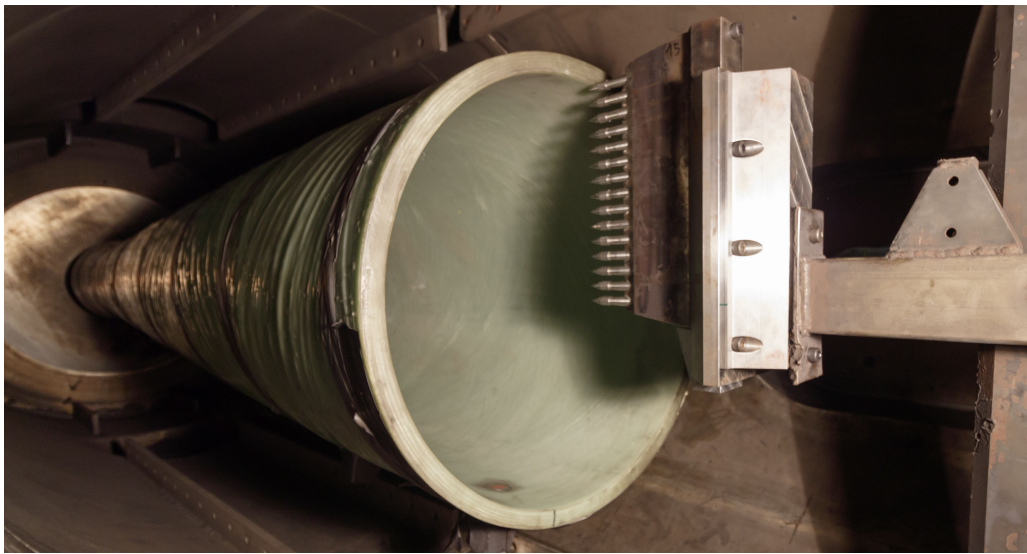
Figure 5.6: X3 expansion tube test section, enclosing Mach 12 nozzle and instrumented rake with conehead sensors.
