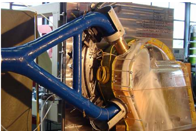
Figure 2 Experimental visualisation of the flow in the casing of a 2-jet Pelton model turbine, Hydraulic laboratory of Andritz Hydro, Switzerland
