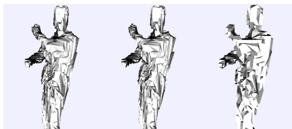
Fig. 4: Original mesh (left) and decoded meshes at 8 (middle) and 6 (right) bit per vertex
