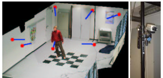
Figure 1: The figure on the left shows an example seven-camera setup used in our system. The red spheres denote camera positions and their viewing directions are shown as blue lines. The image on the right shows one of the video cameras used.
