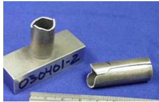
Fig. 11 Interfacial failure mode of “as-consolidated” H13 steel deposited on wrought H13 steel substrate after a bonding strength test
