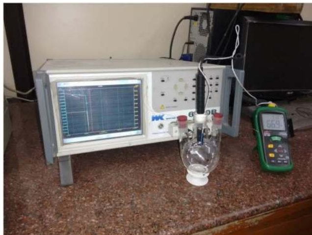
Figure 1. Experimental set-up designed for ammonia sensing using metal oxide-rGO composites.
