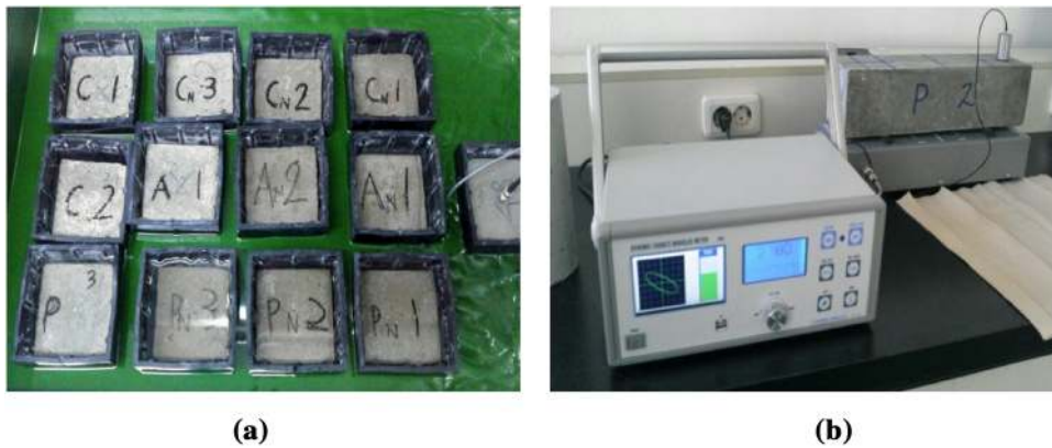
Fig. 6 Apparatus for measuring properties in freeze-and-thaw tests. a Specimens, b transverse frequency apparatus.
