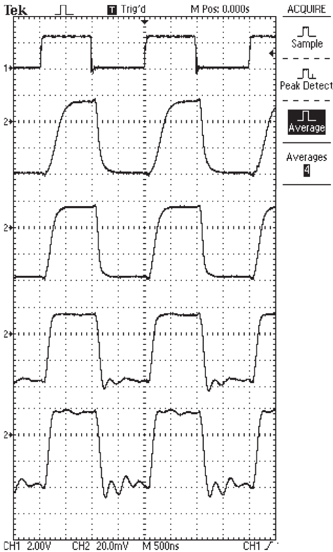
Fig. 5. PSK modulation signal (upper trace) being applied to a 1-W microwave injection signal and the averaged demodulated magnetron output phase (lower four traces) for cathode heater powers of 8, 15, 36, and 43 W in downward order. Corresponding anode currents were 207, 210, 225, and 265 mA. The magnetron operates into a matched load, frequency = 2.4504 GHz.
