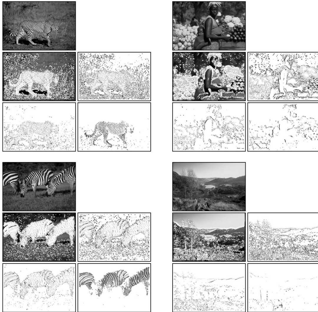
Fig. 4. Example images and their frequency-classified layers. A white color indicates that the pixel is absent from that position.
