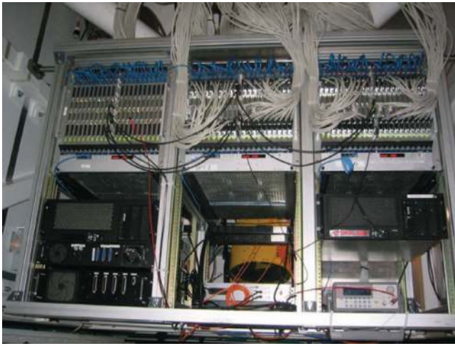
FIG. 12. Photo showing the three readout electronics crates (top half of each rack) housing the oscillator/demodulator circuit boards in the cabin of the South Pole Telescope. Control computers, cryogenic housekeeping, timing, and network electronics are also visible in the bottom half of the racks.
