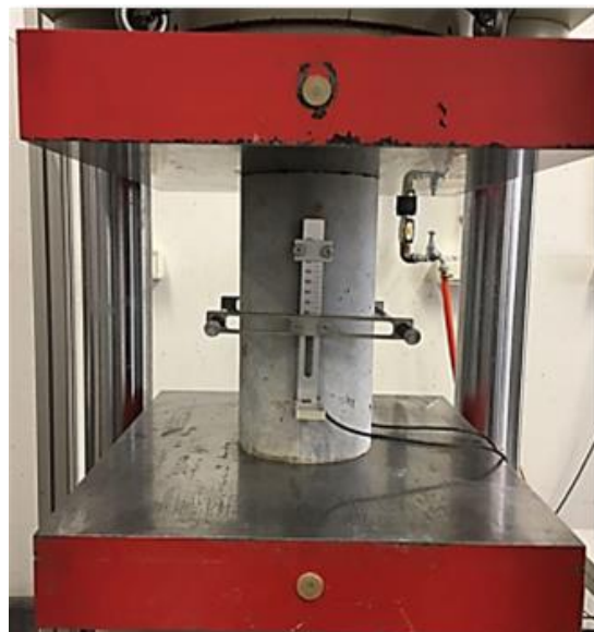
Figure 2. Modulus of elasticity test: strain gauge set up.
