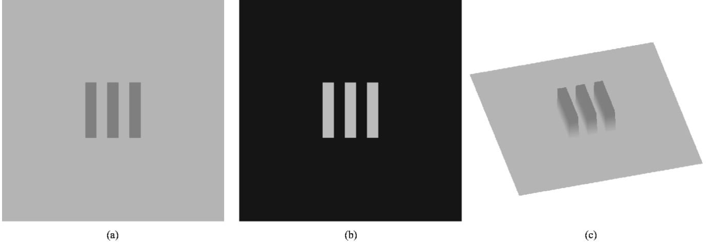
Fig. 3. (a) Amplitude and (b) phase of the test target. The bars width is 256 \mu\text{m} . The sampling step is T = 10 \mu\text{m} and 512 \times 512 samples are evaluated. The amplitude is equal to 1 (dark grey) or \sqrt{2} (light grey). The phase is equal to 0 (black) or \pi/4 (light grey). (c) Perspective view. The grayscale is representative for the amplitude and the elevation for the phase.
