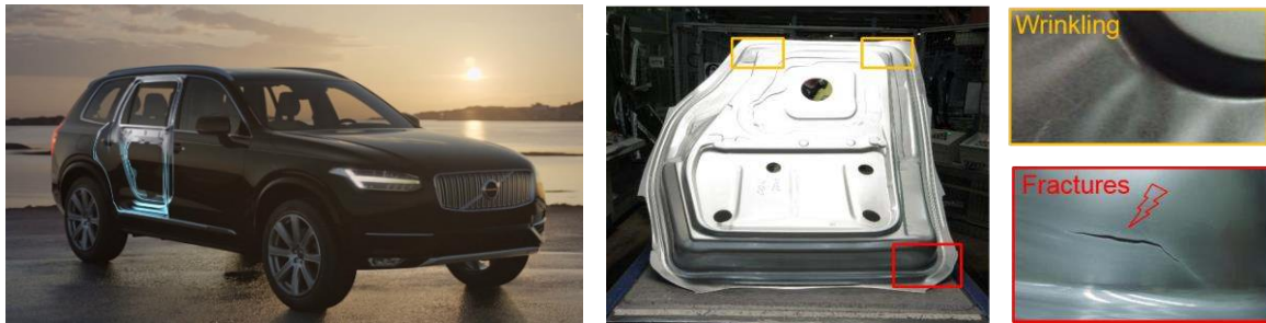
Figure 2. Right rear door inner highlighted in the Volvo XC90 (left) and potential areas of quality issues like wrinkling and splits in production (right)
