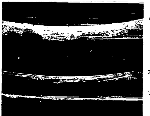
c—Wear plate. Track 1 is wider and has more slider metal deposited on it than do tracks 2 and 3. Tested at 25 revolutions and 760 torr (track 1), 10^{-4} torr (track 2), and 10^{-8} torr (track 3).
