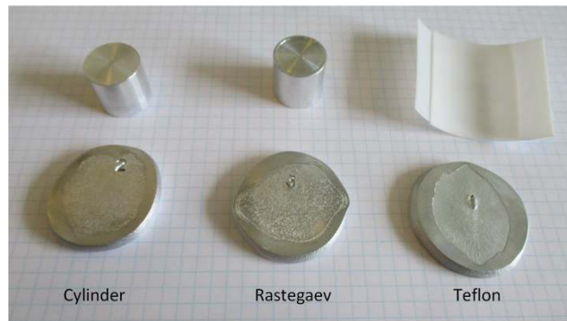
Fig. 2 Compression test specimens before and after deformation
